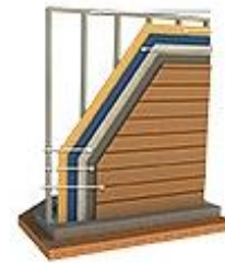
Light Steel Frame
